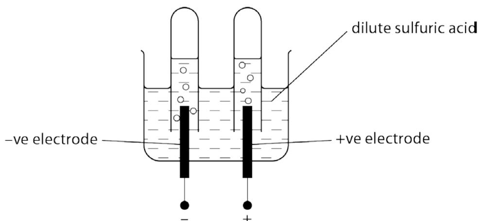
Hydrogen is made at the negative electrode.
