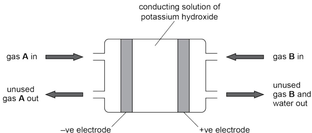
A fuel cell produces electrical energy.
