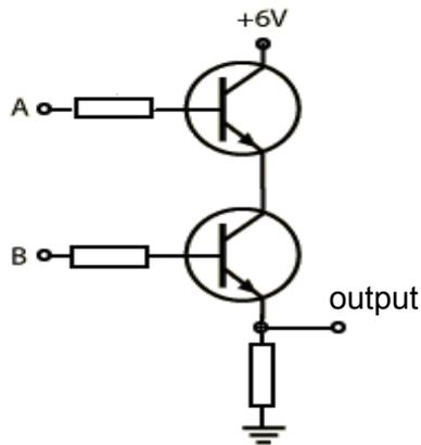
What type of logic gate is shown in the diagram?
