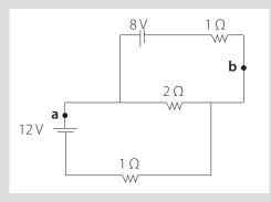
In the circuit above, find the current through the 2 ohm resistor and the potential difference between point a and b.
