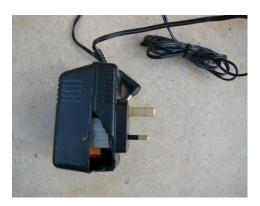
The case is broken exposing live components – risk of fire or shock.
