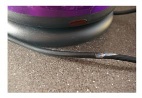
The insulation is damaged on the cable.
