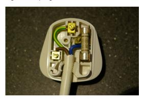
The live and neutral wires have been transposed.
