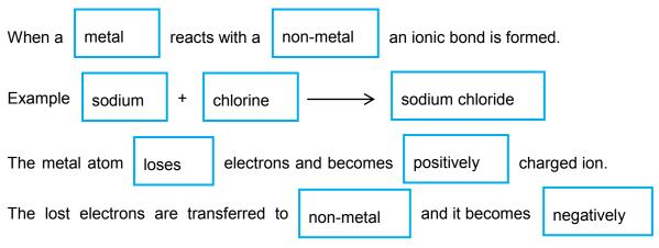
charged ion. Consider the reaction between sodium and chlorine.
