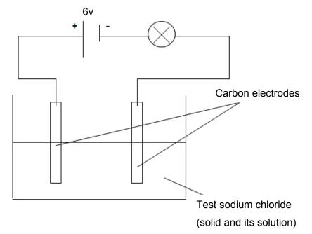
Dip carbon electrodes into some solid sodium chloride.
