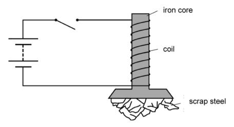
When the switch is closed, the scrap steel is attracted to the electromagnet.
