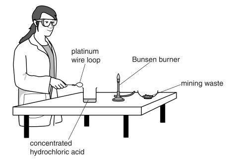
For the flame test she uses a platinum wire loop, a Bunsen burner and a beaker of concentrated hydrochloric acid.
