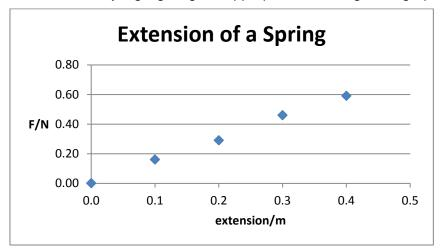
To find Hooke's constant the gradient of the line needs to be calculated. In Excel the gradient can be found by right-clicking on the line and adding a "trendline". The equation can then be displayed on the chart. In this case y=1.48x+0.004. The value in front of x is the gradient and hence the Hooke's constant is  $k=1.48 \, \text{Nm}^{-1}$
