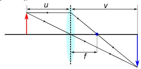
A converging lens is used to produce a magnified image, calculate the image distance v using the equation
