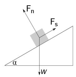
As the object is at rest, the sum of all forces must be zero. To find the magnitude of  $F_n$  and  $F_s$  we need to find the components of w parallel and perpendicular to the inclined plane. A force diagram can then be drawn.
