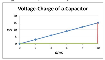
To find the energy stored the area under the curve has to be found. Since the graph is a straight line, a single trapezium can be drawn. The area of the trapezium is given by
