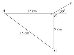
A uniform right-angled triangular lamina ABC with sides AB = 12 cm, BC = 9 cm and AC = 15 cm is freely suspended from a hinge at its vertex A. The lamina has mass 2 kg and is held in equilibrium with AB horizontal by means of a string attached to B. The string is at an angle of 30° to the horizontal (see diagram). Calculate the tension in the string. [4]
