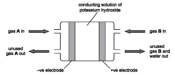
A fuel cell produces electrical energy.
