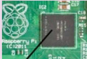
The Raspberry Pi does not have a separate **CPU (Central Processing Unit)**, **RAM (Random Access Memory)** or **GPU (Graphics Processing Unit)**. Instead they are all squeezed into one component called a **System on Chip or SoC unit**. This is essentially the entire computer on one chip.
