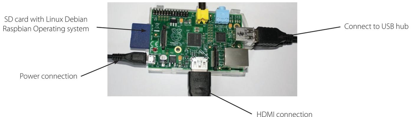
Additionally, the supply voltage required by the Raspberry Pi is 5v DC. The more peripherals that are connected that are drawing power directly from it i.e. that do not have their own power supply, reduce that voltage. If the Raspberry Pi's voltage drops below 4.75v, the system may become unstable. Hardware system designers need to think carefully about how optimum power can be supplied: too much will damage delicate circuits; too little will cause the system to malfunction or not work at all.
