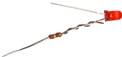
2. Push both the anode (longer lead) of the LED and the other end of the resistor into each of the jumper wires.
