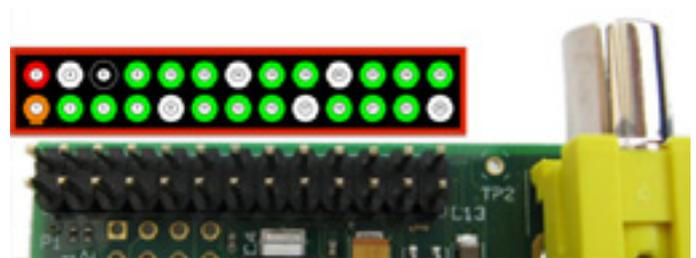
*Raspberry Pi GPIO header pins. The diagram above the pins shows the pin numbers. You will be using pins 3, 5, 7, 17, 20 and 25. **Warning!** You can damage your Raspberry Pi if you do not use the GPIO pins correctly!*
