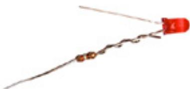
2. Push both the anode (longer lead) of the LED and the other end of the resistor into each of the jumper wires. Repeat this for all 3 LEDs.
