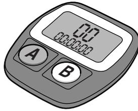
When it is first switched on, the software in the device requires the user to initialise the current time and the circumference of the wheel.
