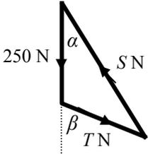
$\frac{S}{\sin 145^\circ} = \frac{T}{\sin 8.5^\circ} = \frac{250}{\sin 26.5^\circ}$ <p><math>S = 321.4</math></p> <p><math>T = 82.8</math></p> | <p>M1</p> <p>M1</p> <p>A1</p> <p>A1</p> | <p>Either Drawing and using a triangle of forces</p> <p>Or Quoting and using Lami's Theorem</p> <p>Correct form of these equations</p> <p>CAO</p> <p>CAO</p> |
