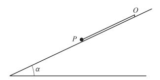
One end of a light elastic string, of natural length 0.3 m, is attached to a fixed point O on a smooth plane that is inclined at an angle  $\alpha$  to the horizontal, where  $\sin \alpha = 0.2$ . A particle P of mass  $m \log$  is attached to the other end of the string. The string lies along a line of greatest slope of the plane and has modulus of elasticity  $2.45m \, \text{N}$  (see diagram).
