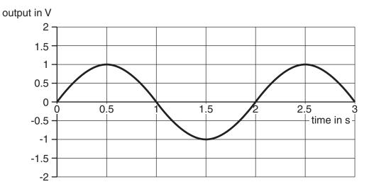
On the graph draw how the output varies when the generator is turned at twice the speed. [2]
