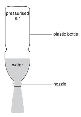
The rocket moves when pressurised air in the bottle pushes water out of the nozzle.
