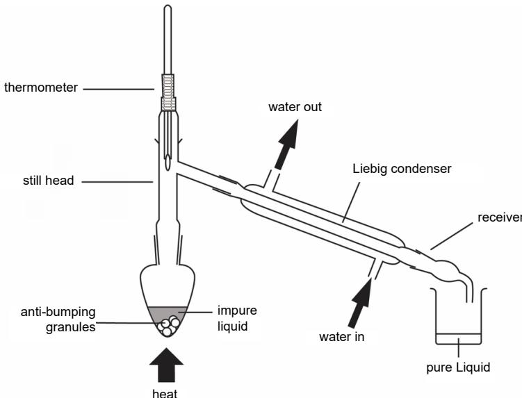
In both distillation and heating under reflux, anti-bumping granules are added to the reaction mixture. These act as nucleation sites for bubbles, ensuring that the liquid boils smoothly.
