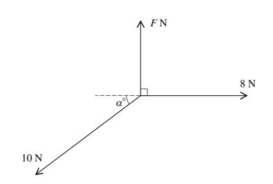
Three horizontal forces of magnitudes F N, 8 N and 10 N act at a point and are in equilibrium. The F N and 8 N forces are perpendicular to each other, and the 10 N force acts at an obtuse angle  $(90 + \alpha)^{\circ}$  to the F N force (see diagram). Calculate
