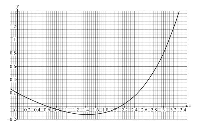
The equation  $0.2 \cosh x - 0.4x = 0$  has two roots,  $\alpha$  and  $\beta$  where  $\alpha < \beta$ , in the interval 0 < x < 3. The secant method with  $x_0 = 1$  and  $x_1 = 2$  is to be used to find  $\beta$ .
