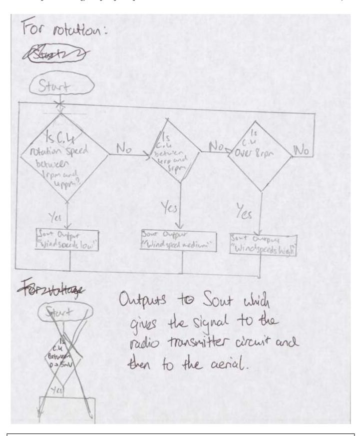
This response clearly shows the method they would use to detect the speed of the wind and the sensor that would be used to do this. They have a clear explanation of how the system would work and have made reference to the output signal that would be produced by the sensor.
