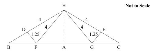
The length of members HE, HG and GE are 4m, 4m and 1.25m respectively. The structure is symmetrical about the centre line, AH, and is arranged in such a way that the area of the triangle in the centre, FHG, is maximised.
