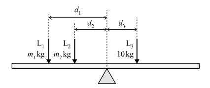
The distance between the fulcrum and  $L_1$  is  $d_1$  m, the distance between the fulcrum and  $L_2$  is  $d_2$  m and the distance between fulcrum and  $L_3$  is  $d_3$  m. Load  $L_1$  has a mass of  $m_1$  kg, load  $L_2$  has a mass of  $m_2$  kg and load  $L_3$  has a mass of 10 kg. The lever has uniform mass which is centred at the fulcrum.
